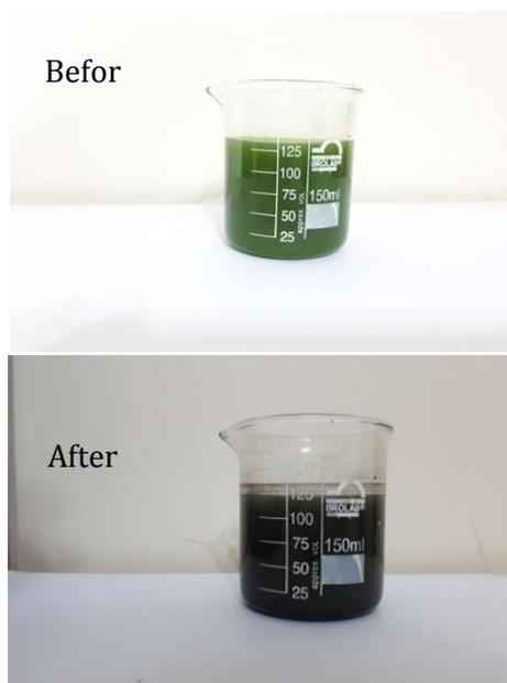
**Figure 1** Color change from green (before adding  $\text{NaNO}_3$ ) to brown (after adding  $\text{NaNO}_3$  and synthesized Ag nanoparticles formation), from ethanolic extract of *S. rebaudiana*
